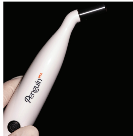
Fig. 1: Penguin® RFA device used to measure implant stability quotient (ISQ) in the present in vitro study.
