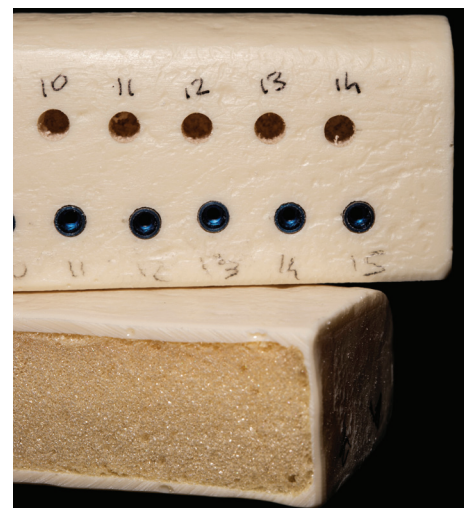
Fig. 2: Polyurethane block (simulated low-density bone) showing the standardized osteotomy sites and representative implants inserted during the experimental procedure.
