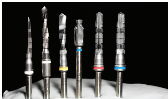
Fig. 3: Drilling instruments used for implant site preparation: (A) Conventional/undersized osteotomy kit (Group OS) and (B) Densah® burs for osseodensification (Group OD).
