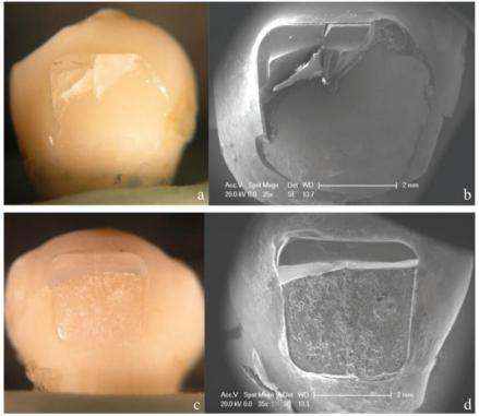
**Fig. 2:** Stereromicroscope and SEM micrographs (35X) of representative failure modes for the experimental groups tested. a,b) show an ARI score 1 from APC FF with 10,000 cycles thermocycling; c,d) show an ARI score 3 from TP with 10,000 cycles thermocycling.
