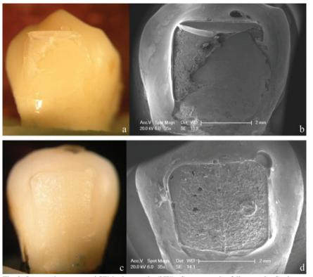
**Fig. 3:** Stereromicroscope and SEM micrographs (35X) of representative failure modes for the experimental groups tested. a,b) show an ARI score 1 from APC FF with 20,000 cycles; c,d) show an ARI score 3 from TP with 20,000 cycles thermocycling.
