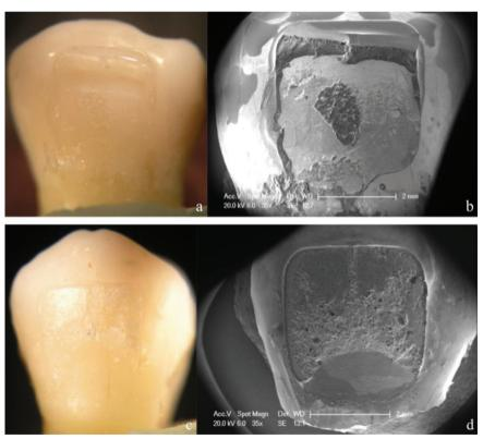
**Fig. 1:** Stereromicroscope and SEM micrographs (35X) of representative failure modes for the experimental groups tested. a,b) show an ARI score 1 from APC FF without aging; c,d) show an ARI score 2 from TP without aging.
