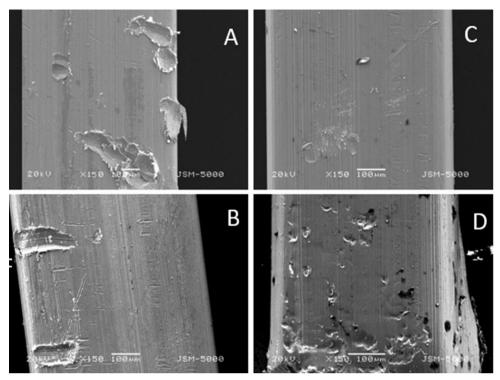
Fig. 4: (A) Group 1: Coated Wire; (B) Group 2: Coated Wire; (C) Group 3: Uncoated Wire; (D) Group 4: Uncoated Wire
