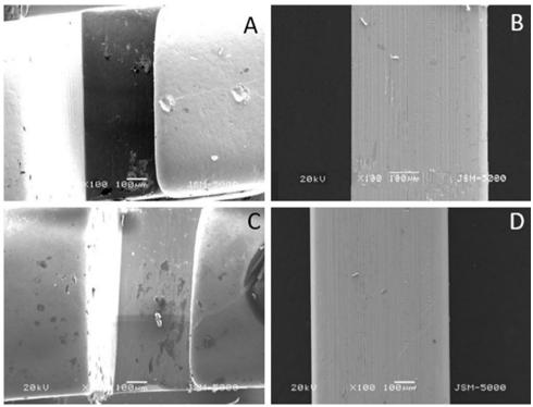
Fig. 2: (A). Coated Bracket before friction; (B). Coated Wire before friction; (C). Uncoated Bracket before friction; D. Uncoated Wire before friction
