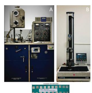
Fig. 1: (A) Vacuum-Coating Unit Model, HINDHIVAC Vacuum-Coating Unit Model no. 15 F6 (Hind High Vacuum Co., Bangalore), helps in producing fine uniform, pure film coating of various metals; (B & C) Metal plates with testing apparatus- (B) central incisor brackets mounted on metal plates and (C) universal testing machine is used for checking frictional resistance
