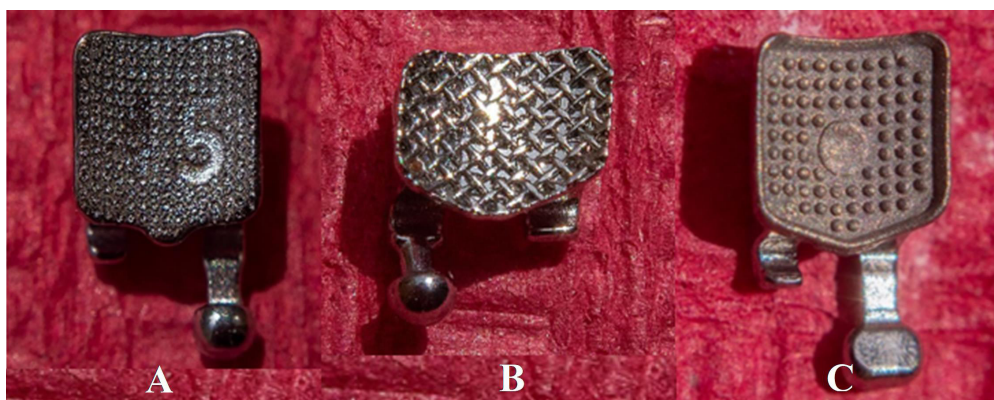
Fig. 2: A: laser-structured base, B: mesh base, and C: base with retaining grooves.
