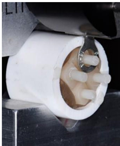
Fig. 1: Block mounted in universal testing machine. Resin cement button loaded in shear at the resin cement/lithium disilicate interface.
