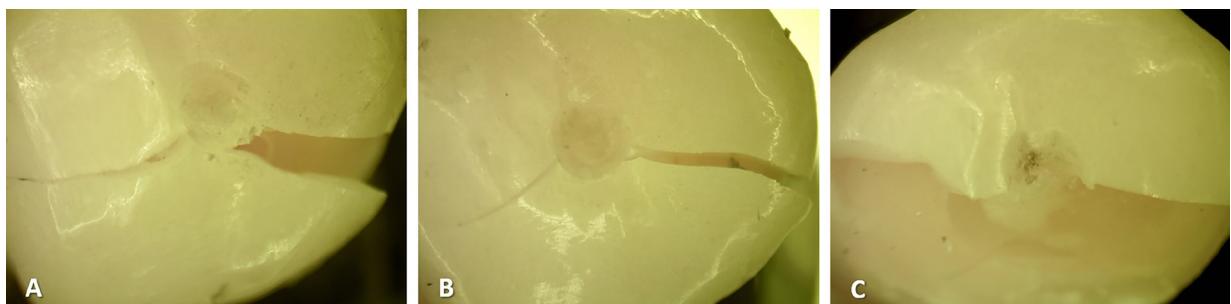
Fig. 4: Evaluation of the type of failure according to the adhesion surface with a stereomicroscope. A: Enamel only (Type 1), B: Enamel-dentin (Type 1), C: Enamel-resin coating (Type 1).
