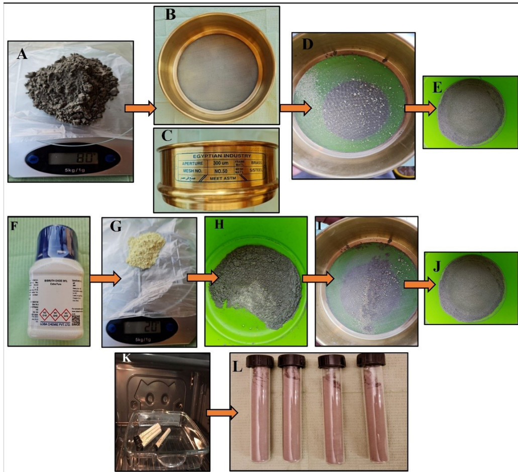
Fig. 1: Preparation of Portland cement for dental use: A) 80 grams of industrial grey Portland cement, B,C) 300 µm sieve, D,E) Grey Portland cement passed through a 300 µm sieve to eliminate large particles, F,G) Twenty grams of Bismuth oxide radio-opacifier were weighed, H,I) Adding Bismuth oxide radio-opacifier to the grey Portland cement and sieving them together to properly mix powder particles, J) Final Portland cement/Bismuth oxide powder mixture K) Placement in heat resistant glass tubes and sterilization in a hot air oven of 170 °C for 1 hour, L) Storage in heat resistant glass tubes.
