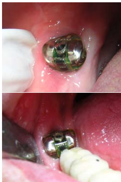
Fig. 3. Clinical view of the miniature electro-stimulator supported by a dental implant located in the third molar area.
