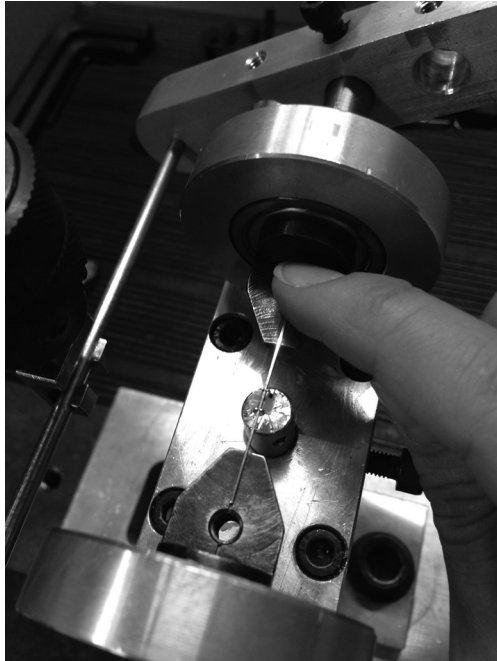
Fig. 1: Universal testing machine with the wire-bracket system positioned for torsion test.
