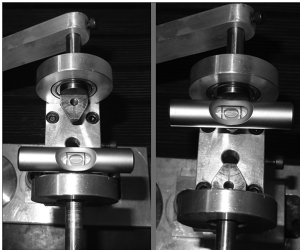
Fig. 2: “Bubble Level” accessory to leveling the system in each start test.
