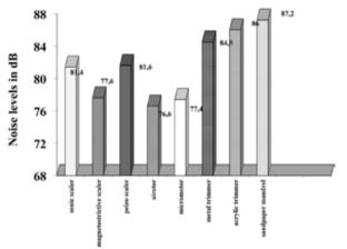
Fig. 2. Noise levels of dental equipments measured at 6 inches from the operator's ear.
