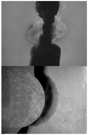
Fig. 4. Failure modes observed (a) IPN post fracture; (b) cross-linked post composite debonding.
