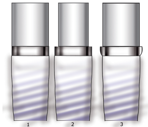
Fig. 1. Implant-abutment options: in number 1, the joint between components with an equal diameter. However, in the following examples it is modified (platform switching). In number 2, the restoration diameter is reduced and in number 3, the implant platform is expanded, matching implant and abutment diameter.
